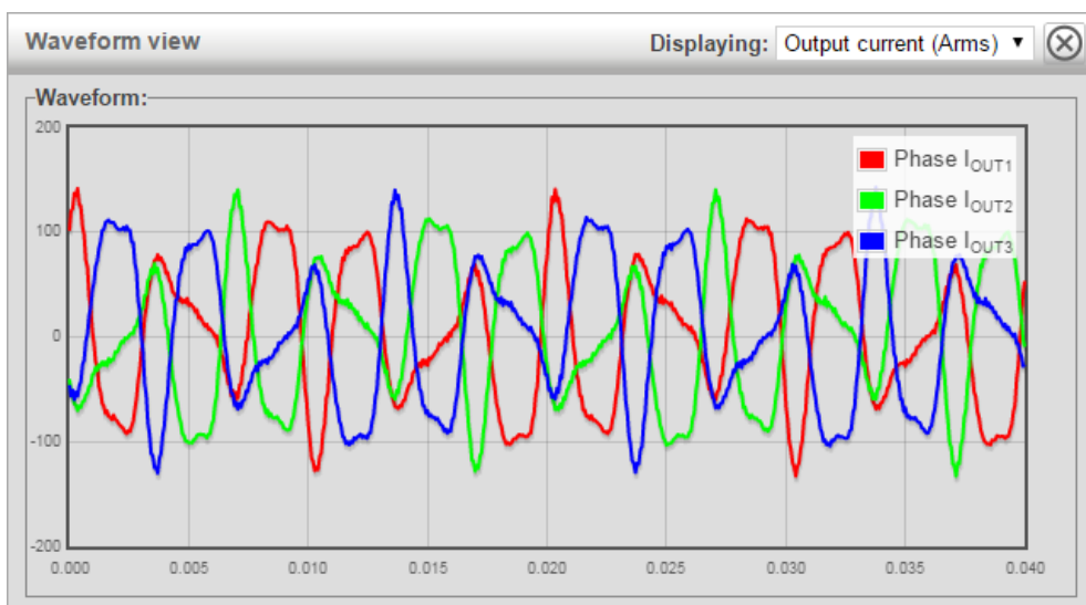
Figure 25: Waveform view window showing Compensation current
