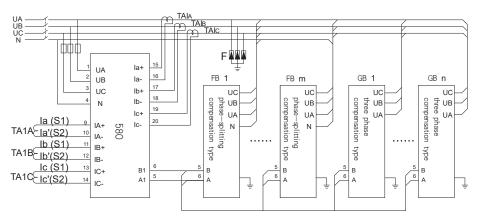
Note: In single-phase sampling, the primary CT of distribution only needs to be connected to terminal 9 and terminal 10 of phase A of distribution current.
