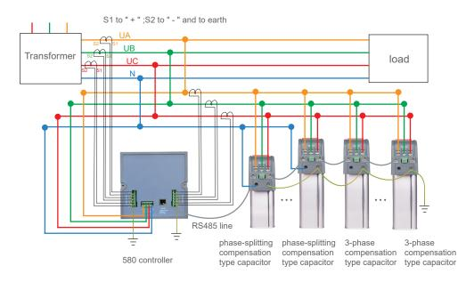
Note: The primary CT ratio of the distribution current must be set, for example: 500/5, set to 100.
