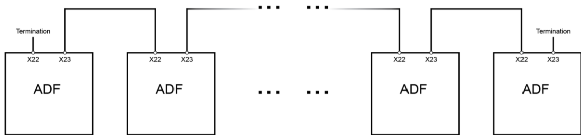
Figure 18: Example setup for Multi-master operation
