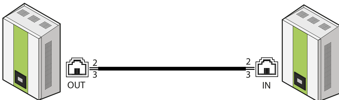
Figure 27: Connecting 2 devices in parallel, using the communication cable.
