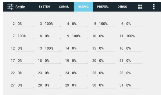
Figure 6-9 2 nd to 50 th harmonic compensation ratio setup
