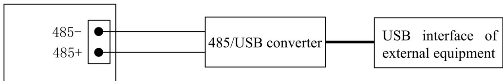
Figure A4-2 Wiring of 485 communication interface and serial port of external equipment
