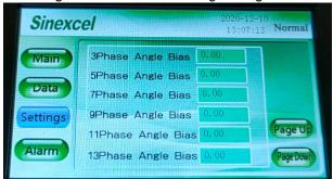
Phase angle calibration can be set-up for a few selected harmonics. Values are probably in radiant.
