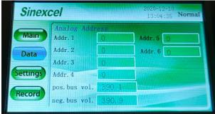
In stopped mode, the DC-link voltage is charging up to 2x 330 V = 660 V. That indicates that the two levels of the pre-charge are feed by two independent pre-charge circuits. Each connected phase-neutral.
