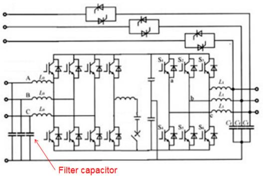
The topology of high frequency UPS and filter capacitor in the inputside is as below shows:
