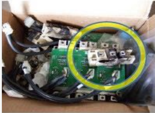
VFD Premature Failure
