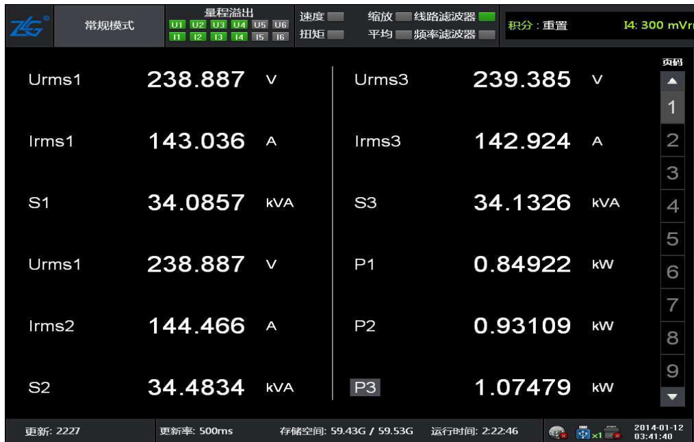
效率测试图 (效率: 97.22%) Efficiency test chart (efficiency: 97.22%)
