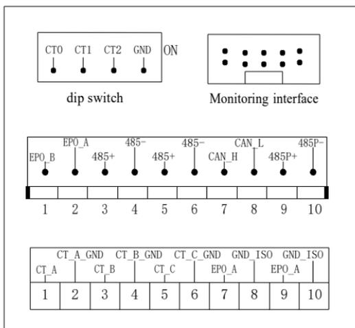
Figure 2-4 Interfaces of external CT terminal strip
