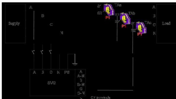
Figure 2-2-1 Wiring of single power module (3-phase 4-wire system)
