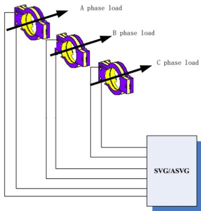
Figure 2-5 CT installing direction diagram
