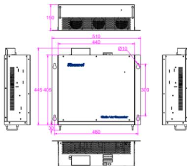
Figure 2-1-2 SVG15/30 wall-mounted LED
