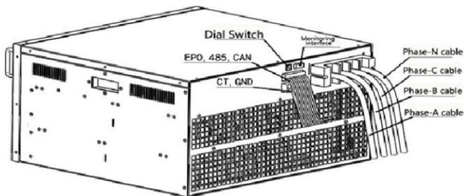
Figure 2-3 Wiring diagram of SVG single power module
