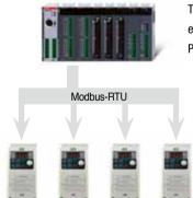
The optional modbus communication enables controlling drives through PLC and other controlling devices.
