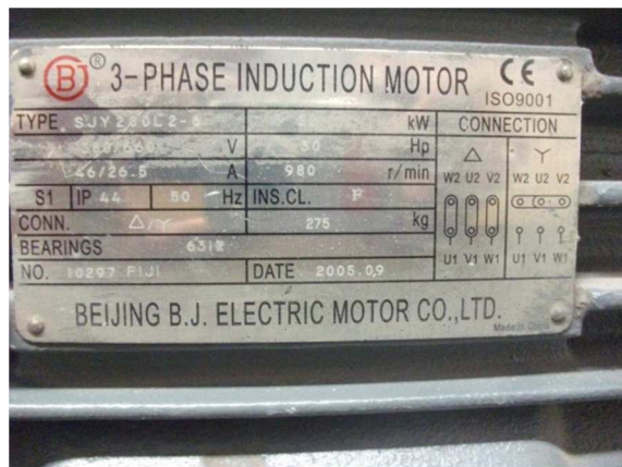
Auxiliar Equipment: Motor BEIJING type B.J 22kW s/n:10297FIJI detailed plate.
