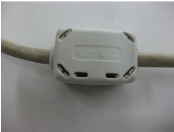
Control cable ferrite Würth Elektronik 742 711 32.
