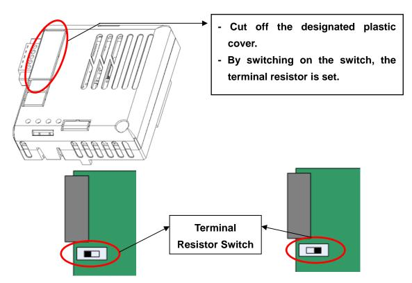
When the switch of terminal resistor is placed in left side (Off)
