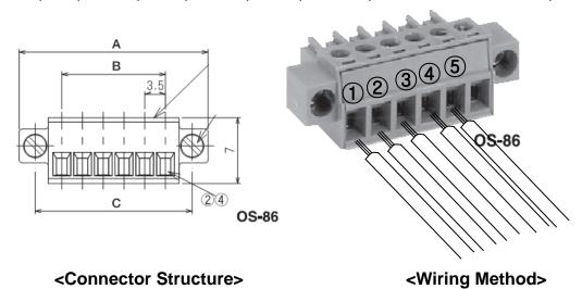
\* Signal connector OSADA OS-86-5P must be used for iS7 CC-Link communication option module. (5-Pin connector)
