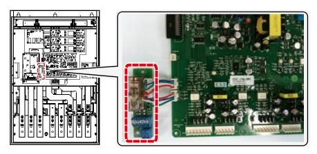
Refer to the following figure and install the safety board to the main SMPS board of the inverter using cable connectors.
